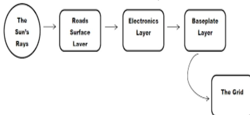
**Fig.4. Flow chart showing the complete process of working of solar roads.**
