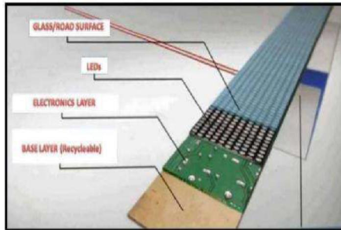
Figure 4: Construction Layers Solar Roadway
